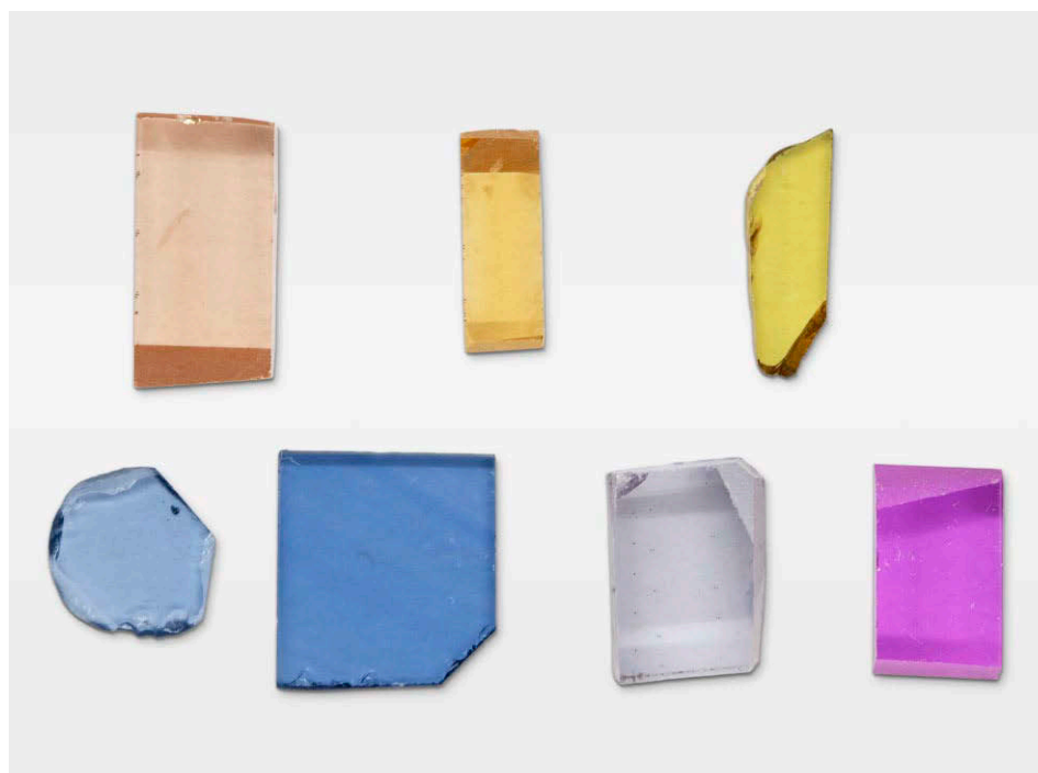
Figure 2. Shown are some of the many crystallographically oriented samples used in this study. Clockwise from top left, they represent the following chromophores: h^{\bullet}\text{-Cr}^{3+} , h^{\bullet}\text{-Fe}^{3+} , \text{Fe}^{3+} , \text{Cr}^{3+} , \text{V}^{3+} , and \text{Fe}^{2+}\text{-Ti}^{4+} (the two blue samples at lower left). The sample in the far lower left corner is a natural blue sapphire from Yogo Gulch, Montana, and the sample in the upper right corner is a natural yellow sapphire from the Subera deposit in Queensland, Australia; the rest are Czochralski grown. Sample numbers clockwise from upper left are 991, 992, 1121, 1110, 1102, 1065, and 1014; detailed information on the samples can be found in Appendix 1.
